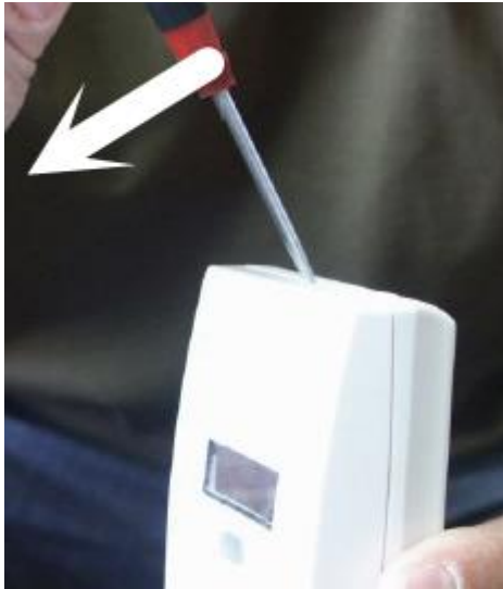
Figure 2. Closed housing seen from the side. The housing is opened by inserting a screw driver and pushing left (to the front side). The locking hooks will then be released.
